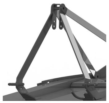
Connect your lower lift arms on the rear of the tractor to the hitch pins on the lower outside part of the hitch. The top link will then connect to the upper swivel bracket for pitch control. Lengthen or shorten your top link by turning the turnbuckle to make the brush cutter parallel to the ground.
